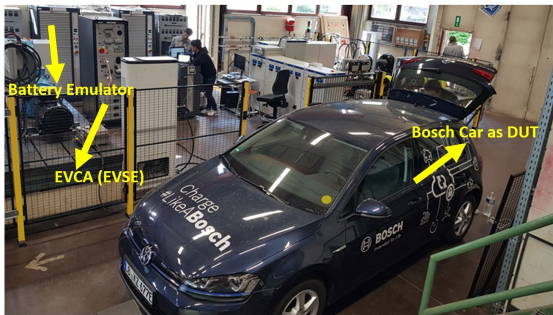
Figure 9. Experimental setup for V2G test with BOSCH passenger car.
